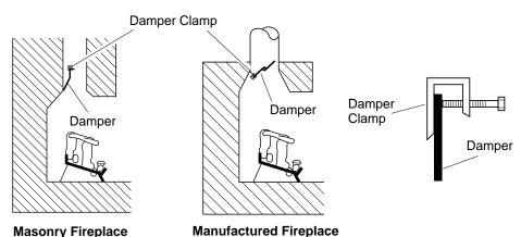
Masonry FireplaceManufaFigure 10 - Attaching Damper Clamp
